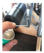
6. Clean the boreholes in the adapterplate and the bolts included on the adapter with loctite 7649.
