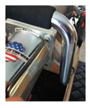
8. Place the adapter, with the sticker to the front and tighten the bolts securely.
