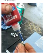
7. Place two rings on each bolt, with the convex side up. Add Loctite 243 on each bolt.
