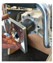
4. Place the adapter plate (only for adapter 301405, 301403 and 301415) with the ingrained edge to the machine.
