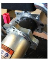
2. Turn loose the bolts with included allen key and remove the chuck.
