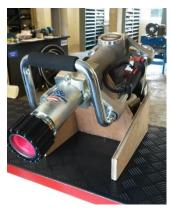
1. Place the machine firmly down. Remove the Locking nut and adapter from the chuck.
