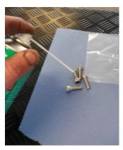
3. Clean the new adapterplate bolts and the boreholes on the machine with Loctite 7649.
