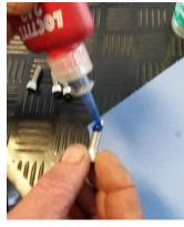
5. Add Loctite (Loctite 243) on the bolts and place bolts. Tighten the bolts securely.
